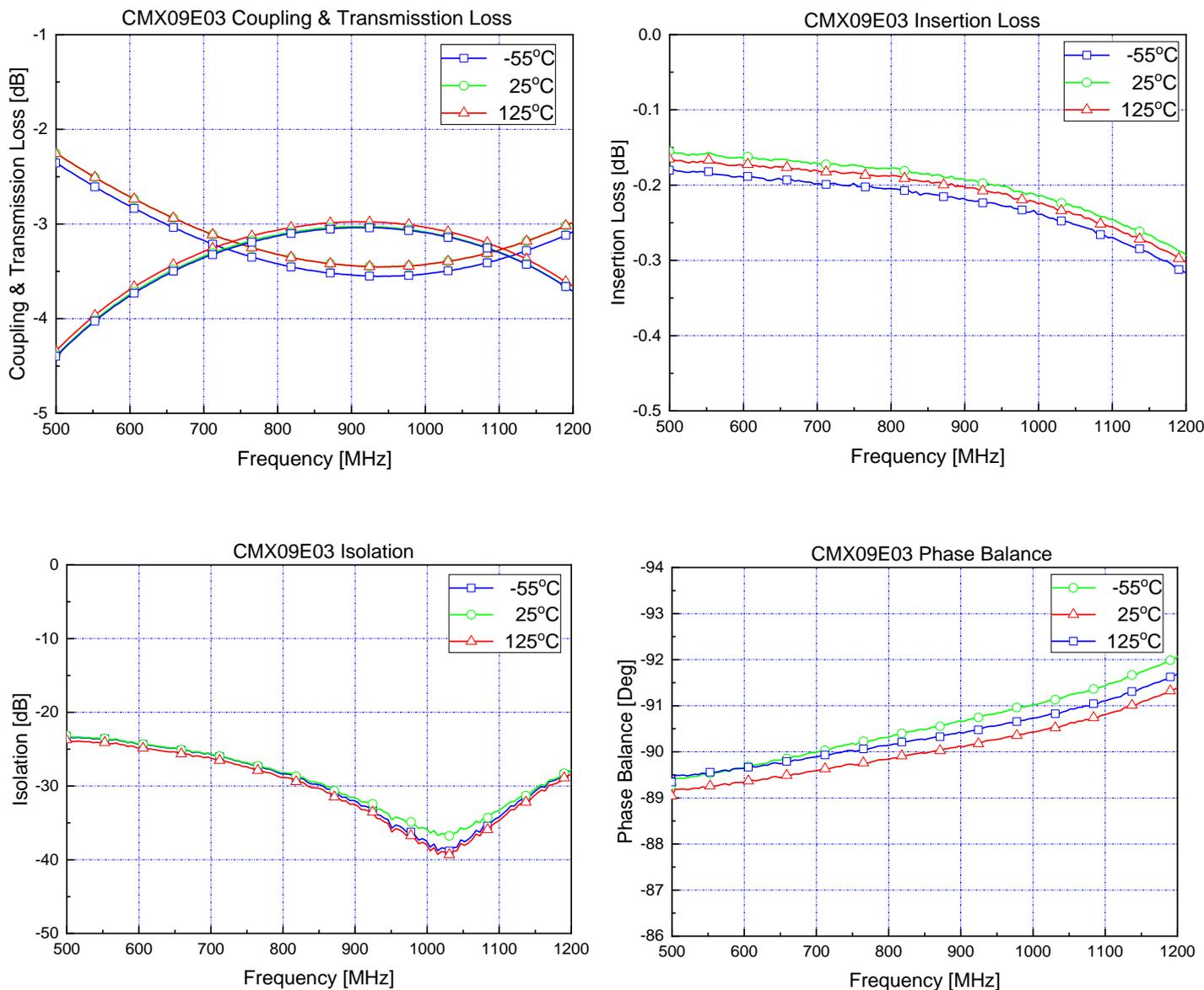
**Figure 4. Test Plots of Coupling and Transmission Loss, Insertion Loss, Isolation, and Phase Balance (-55 °C, 25 °C, and 125 °C)**
