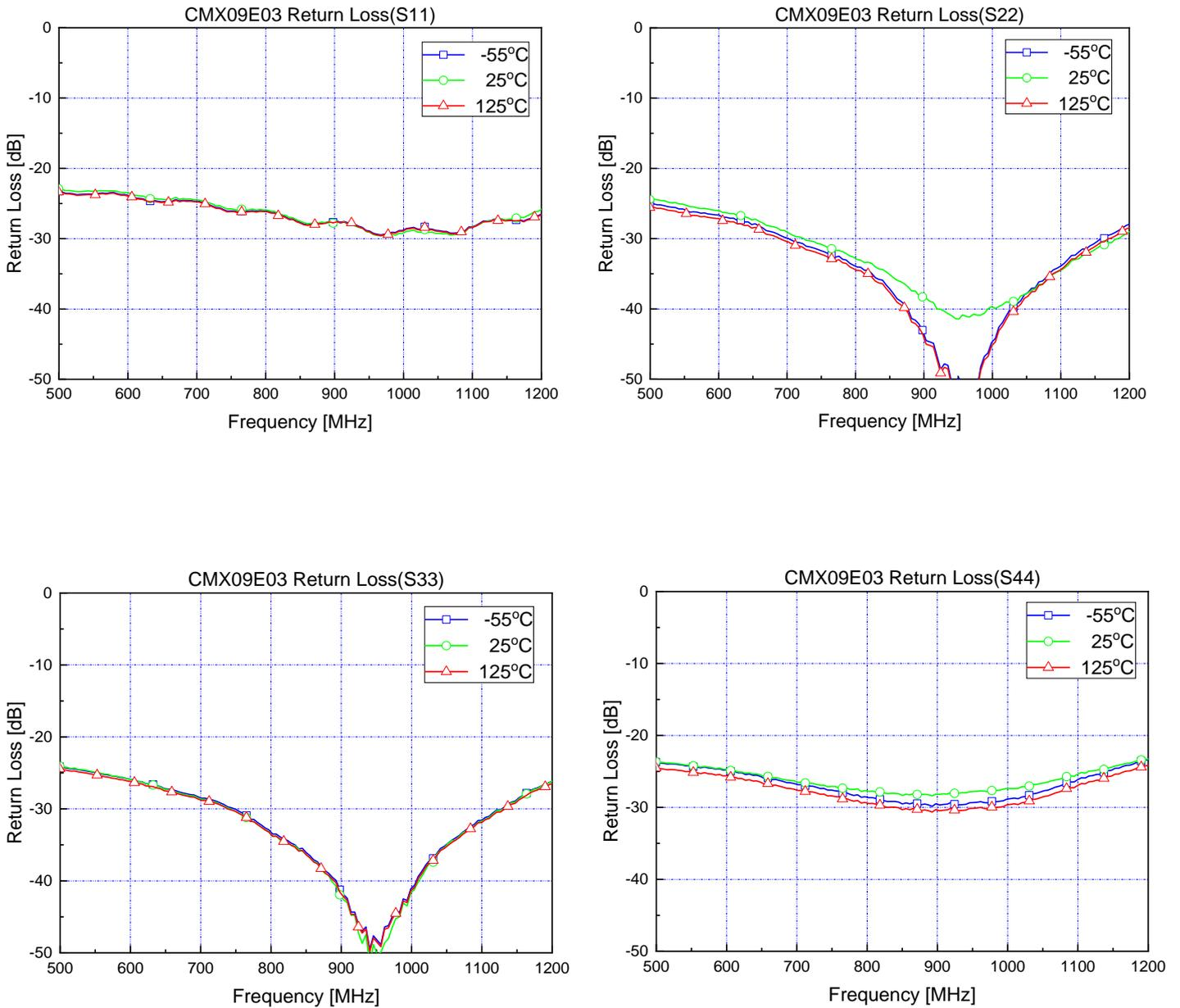
Figure 3. Test Plots of Return Loss (-55 °C, 25 °C, and 125 °C)
