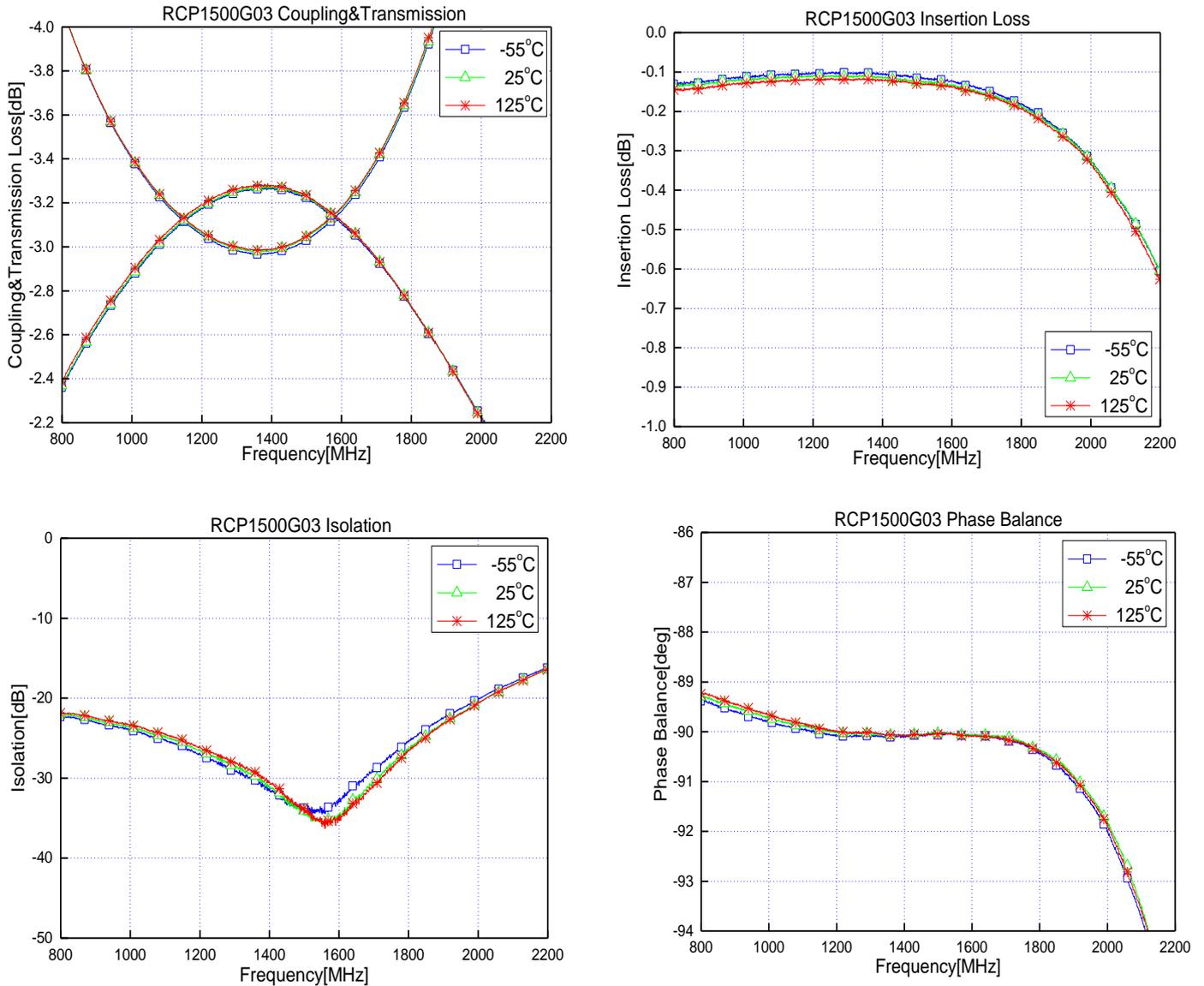
**Figure 4. Test Plots of Coupling and Transmission Loss, Insertion Loss, Isolation, and Phase Balance (at -55 °C, 25 °C, and 125 °C)**
