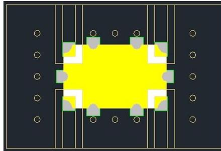
**Figure 11. Placing the RCP1500G03 on the 11 Points of the PCB Surface**
