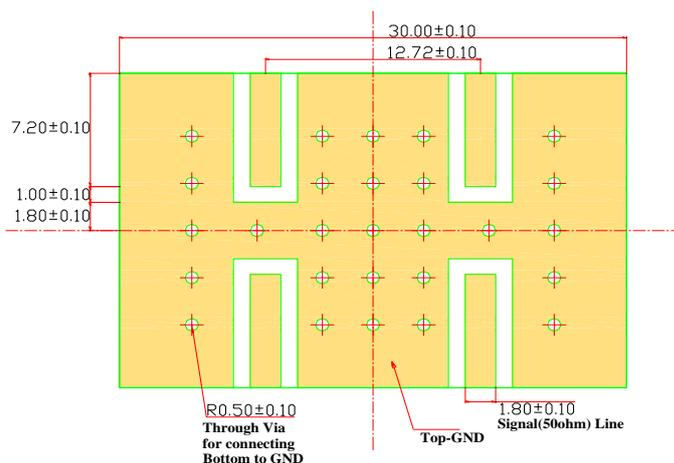
**Figure 6. RN2 Technologies Test Board Layout**
